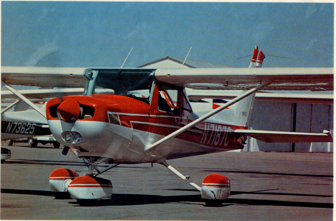
Altered shape of the nose and a longer exhaust pipe are two clues that there's something new under the cowl. Photos by author.
